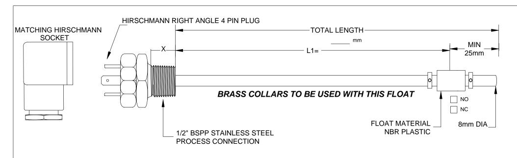
STANDARD - NO or NC CONTACT RATED AT 32V AC/DC @ 500mA RESISTIVE LOAD
